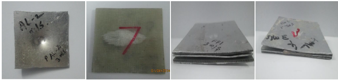
Fig 4. (a) Monolithic aluminium (b) Glass fiber reinforced composite (c) Fiber metal laminate (d) Fiber metal laminate with filler at velocity 3m/s
