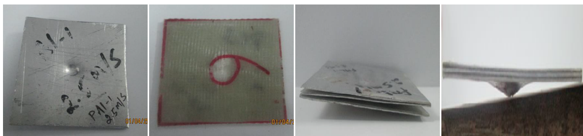
Figure 3. (a) Monolithic aluminium (b) Glass fiber reinforced composite (c) Fiber metal laminate (d) Fiber metal laminate with filler specimens at velocity 2.5m/s
