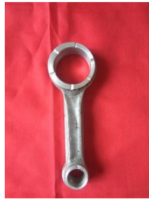
Fig 5. Finished connecting rod squeeze casted composite
